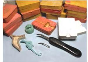
The #11 blade is triangle shaped, and the #12 is hawksbill shaped. I find the hawksbill is particularly nice for cutting the registration keys of the mold.
