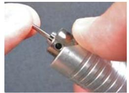
So I have two ways to speed up that task. For opening up the jaws, I just remember "four," the number of turns I have to make to open the chuck just enough from the 3/32-bur shaft size to the larger 1/8-bur shaft size.
