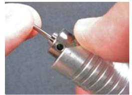
So I have two ways to speed up that task. For opening up the jaws, I just remember "four," the number of turns I have to make to open the chuck just enough from the 3/32-bur shaft size to the larger 1/8-bur shaft size.
