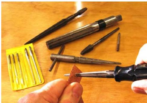
Other times when I'm drilling a hole for riveting and can't find the exact-size drill, I simply drill the holes with a slightly smaller bit and enlarge them with a reamer until the wire just fits.
